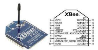
Figure 2: X-Bee Pro modules and Pin outs
